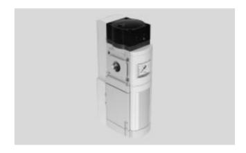
The electro-pneumatic soft-start and quick exhaust valve is used to reduce pressure quickly and reliably and to build up pressure gradually in industrial pneumatic systems and terminals.
