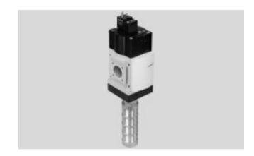
Electro-pneumatic soft-start and quick exhaust valve for gradual pressurisation and quick exhausting of system components (single channel). The main flow control valve in the end cap permits a gradual build-up of output pressure p2. Once the output pressure p2 has reached the set pressure switchover point (switching pressure), the valve opens and the full operating pressure p1 is present at the output.
